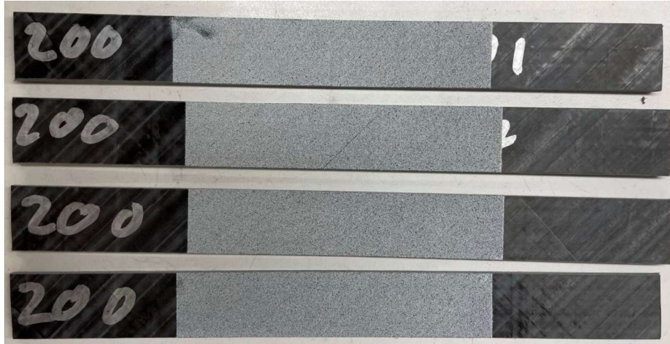
Figure 2 – ASTM D3039 tensile specimens with speckle pattern for DIC strain measurement
